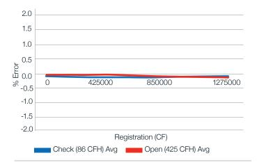
The accelerated life test of the Intelis 425 Gas Meter is stable and the Open (425 CFH) and Check (86 CFH) track tightly.
