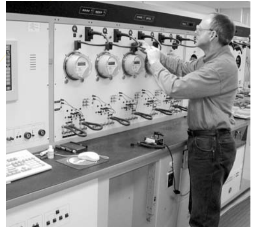
The CENTRON meter's improved performance, such as low starting watts and low burden captures energy that was not monitored in the past by electromechanical meters.
