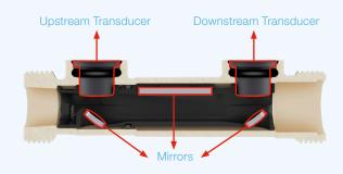
Physical principle: Propagation of acoustic waves in a liquid
