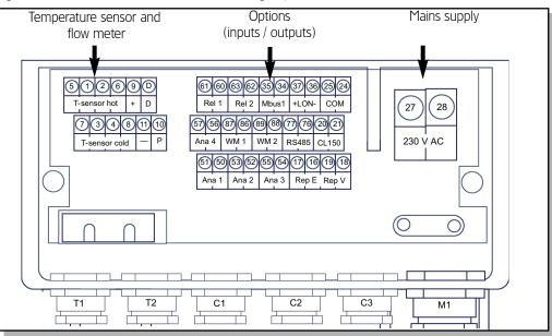
Install all connection cables into lower housing part using the cable entrances and strain relief clamps (where applicable). The indication of cable entrances is as follows:
