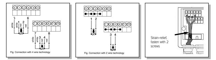
In case of shielded wires ensure a good contact between strain-relief and shield. In general the shielding must be connected on one side of cable only.
