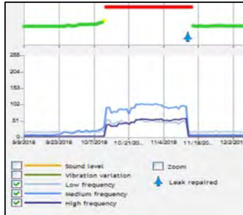
Example of a leak found and repaired during the project
